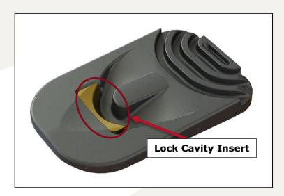
The Lock Cavity Insert is a hardened steel approximately 550 HB. As such to preserve the parts integrity the inserts must be removed prior to any heating or welding processes. Store the inserts in a safe location so that they can be reinstalled after the lip has cooled below 80°C (176°F).
