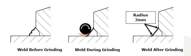
The end of the weld must be tapered and smooth prevent a stress riser at a change in restraint or profile location.
