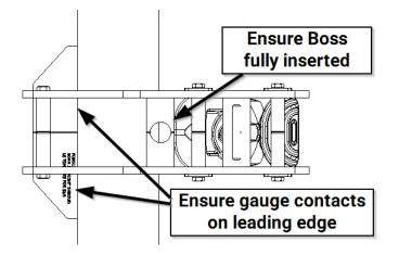
For 50mm lip thickness, the leading edge of the frame is interchangeable with different sized edges matching the widths of the shrouds. This enables you to easily control the gap sizes between the shrouds.
