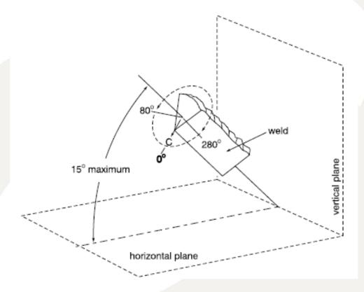
The longitudinal axis of the weld may be inclined no more than  $15^{\circ}$  with respect to the horizontal plan. The centre of the weld face "C" must lie within the rotational limits of  $80^{\circ}$  to  $280^{\circ}$  as shown.
