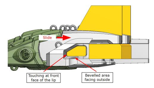
Fix the Front Split Lip End Cap position in place with one 12mm / 1/2'' long tack weld at the root of the weld prep.
