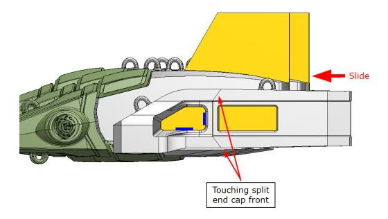
Make a12mm / 1/2'' long tack weld at the root of the weld prep to secure the Back Split Lip End Cap position in place.
