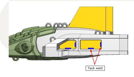
Preheat the lip plate and split end caps area to be welded to 150°C before proceeding with complete weld. Start welding on the area around the Split Lip End Cap as specified in the figure below with a weld size of 20mm to 25mm fillet as shown in detailed in the Welding
