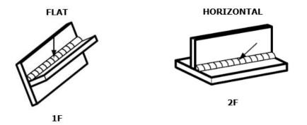
Deviation from the Flat or Horizontal position is permissible as shown in figure below as typically described in welding standard AWSD1.1, Structural Welding--Steel, Figure 4.2 "Positions of Fillet Welds".
