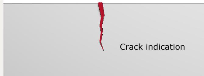
The cracked material must be gouged or machined away sufficiently to permit a full penetration repair weld to be made, with no traces of crack left behind and no new significant defects introduced. In any case, where air carbon arc gouging process is used, at least the final 5mm of material should be removed by grinding. Ensure the channel has a distinct V- or U-shape groove for weld repair.
