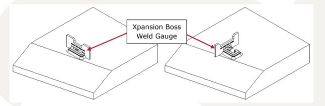
The end of the weld must be tapered and smooth prevent a stress riser at a change in restraint or profile location.
