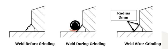
Inspect finished weld size using Xpansion Boss Weld Gauge. This gauge is a simple GO / NO-GO gauge. The gauge should be able to pass easily over the welded Xpansion Boss while maintaining contact with the lip surface. If the gauges interfere with the weld surface continue to grind the weld until the gauge can pass over the Boss.
