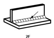
Deviation from the Flat or Horizontal position is permissible as shown in figure below as typically described in welding standard AWSD1.1, Structural Welding--Steel, Figure 4.2 "Positions of Fillet Welds".
