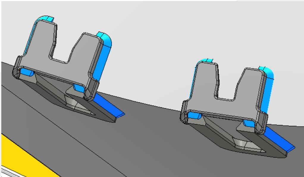
After both boss pieces have been fully welded, inspect again with the Heel Shroud Boss Assembly Gauge.
