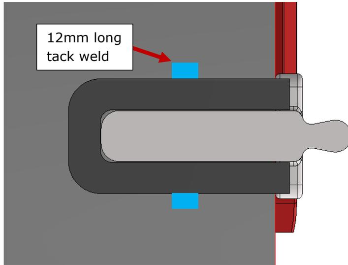
After the first Long U Boss piece has been tack welded, remove the gauge, and displace the second Short U Boss piece until it contacts the first Boss piece. The second Short U Boss piece should also butt against the side of the bucket.
