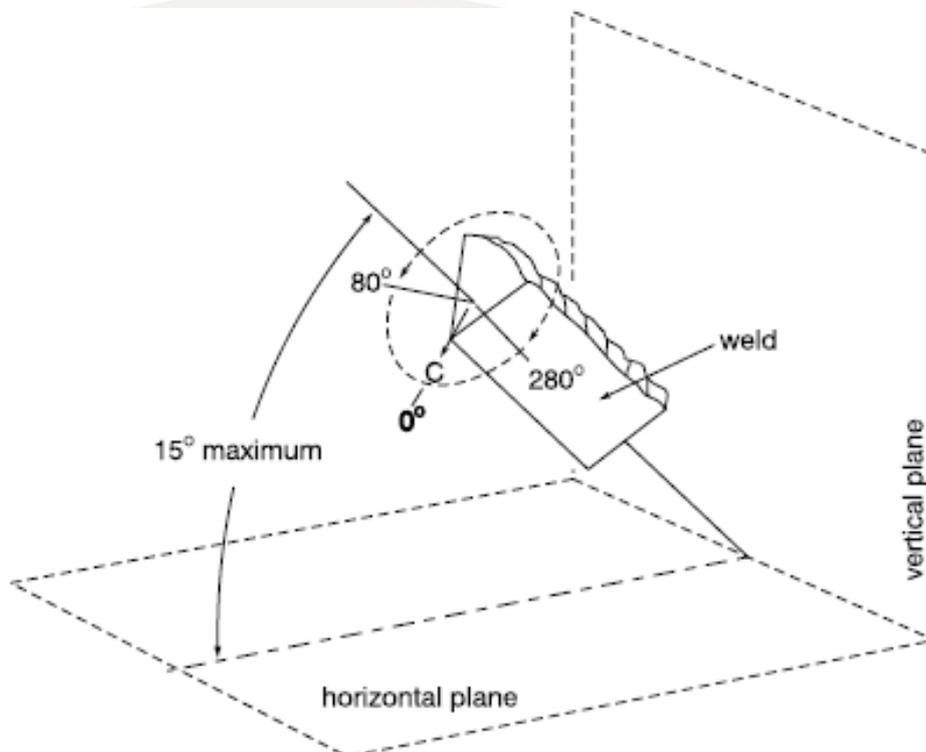
The longitudinal axis of the weld may be inclined no more than 15° with respect to the horizontal plan. The centre of the weld face "C" must lie within the rotational limits of 80° to 280° as shown.
