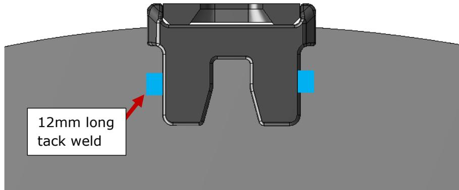
After both boss pieces have been tack welded in place, use the Heel Shroud Boss Assembly Gauge to check that both boss pieces are positioned correctly relative to the bucket as indicated in the figure below. This is done to assure good fitment of the heel shroud with the welded boss assembly.
