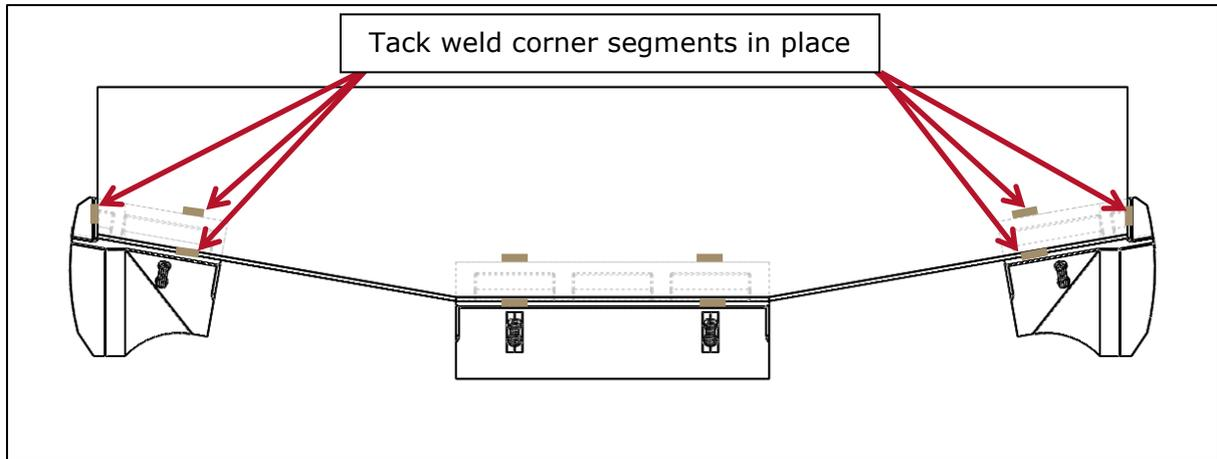
Trim Half Arrow side segments to suit lip. Place Half Arrow side Segments on to lip and tack in place with two 25mm / 1" tack welds on the bottom rear edge and two 25mm / 1" tack welds in the top weld gap.
