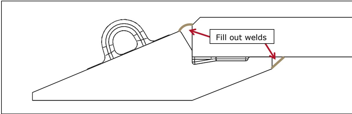
Finish the welding process by welding out the 90mm long weld preparation grooves that run down the face of the Half Arrow Segments.
