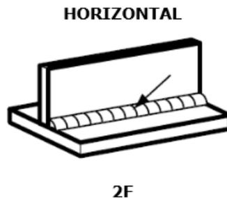
Deviation from the Flat or Horizontal position is permissible as shown in figure below as typically described in welding standard AWS D1.1, Structural Welding--Steel, Figure 4.2 "Positions of Fillet Welds".
