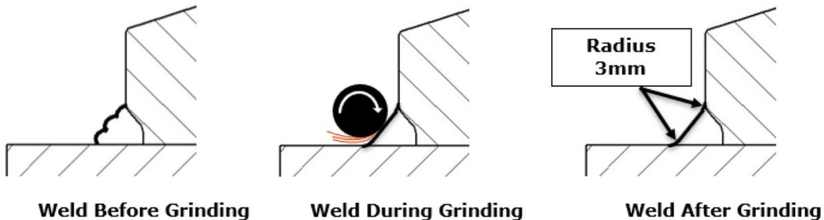
The end of the weld must be tapered and smooth prevent a stress riser at a change in restraint or profile location.
