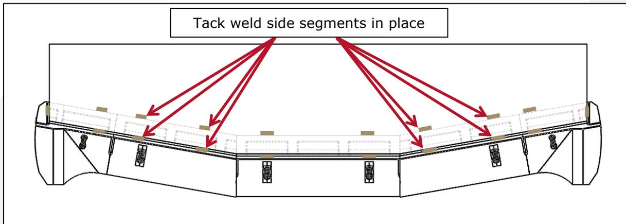
Complete a full root run and one capping pass along in the top weld gap followed by a full root run and one capping pass along the bottom edge of the Half Arrow. Following this proceed to fill out the welds as suits your welding equipment.
